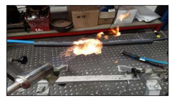
When the sleeve has been shrunk sufficiently adhesive will be showing at the ends,
